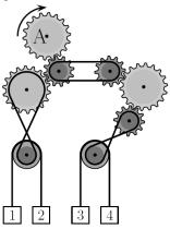
20- The gear marked A is turned clockwise, as shown. Which two boxes will move upwards?
