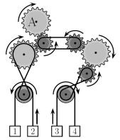
By following the movement of the gears starting from gear A, we will observe the movement as in the following figure, noting that any two adjacent gears will move in opposite directions, and any two gears connected to a belt will rotate in the same direction, and any two gears connected to a
